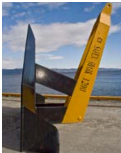
EIVA-SAFEX - Production of anchors and a mooring plate holder which has been developed in cooperation with the Norwegian seafarming industry. The mooring plate holder is a tool which has greatly improved safety when performing maintenance on fish farming installations.
