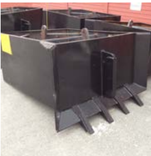
EIVA-SAFEX - Production of anchors and a mooring plate holder which has been developed in cooperation with the Norwegian seafarming industry. The mooring plate holder is a tool which has greatly improved safety when performing maintenance on fish farming installations.
